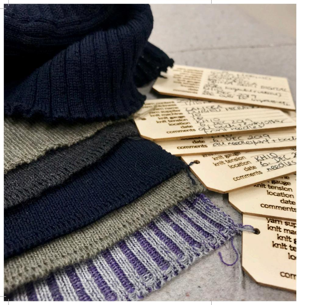
Through the manual knitting process I discovered many nuances that affect both the surface texture and the inner structure of a knitted material; the yarn thickness, the carriage tension, the feeder tension. I have chosen not to write about such details in this thesis, although they were obviously practical considerations in my making and selection process. I will specifically write about my experiences with yarn choice and the stitch type.
