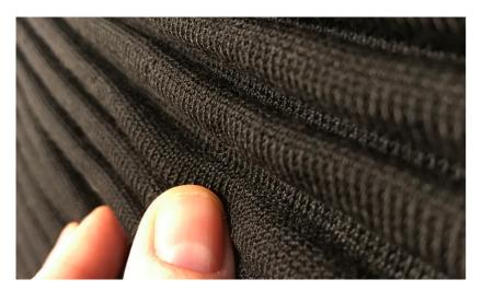
Figure 39: Knitted stimulatory tucks at Ekornes in very hard yarn Figure 40: Knitted elasticated structures at Ekornes in very hard yarn
