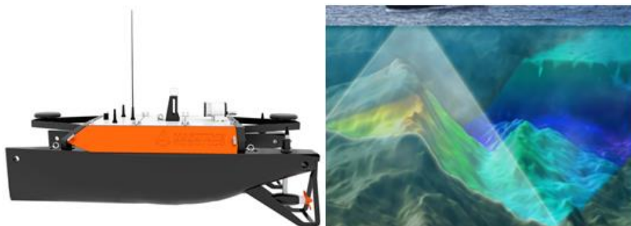
Left: USV Otter (maritimrobotics.com) Right: Visualization of seabed mapping with sonar (dragonfishoffshore.com)
