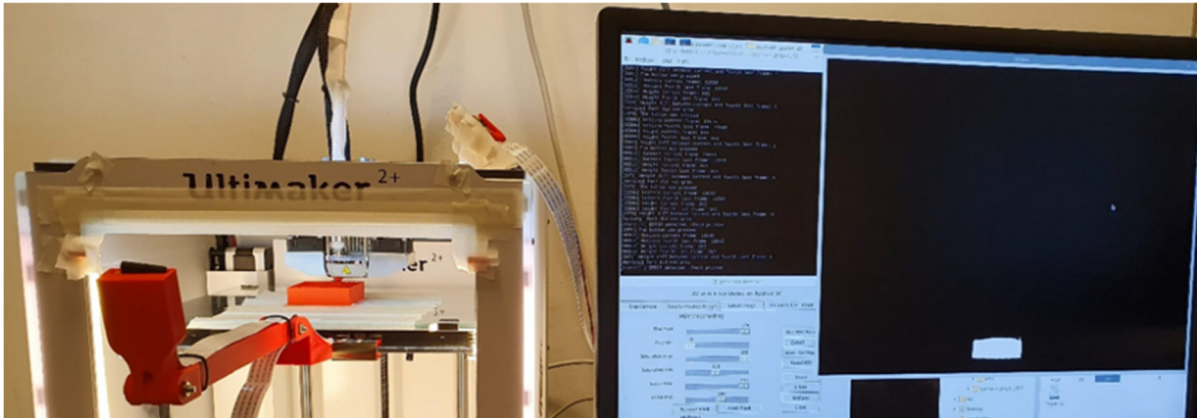
Figure 27 Fast Cube filament runout error
