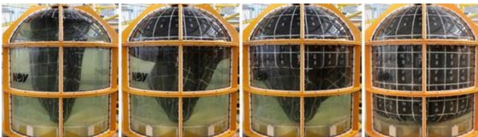
Figure 2.10: The process of filling the bladder in a bladder tank (Equinor, 2019a)
