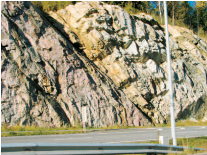
Figure 4.5: Bedrock gneiss in Ås, Norway. This rock mass is an example of class B in the categorization by Klüver and Kveen (2004).
