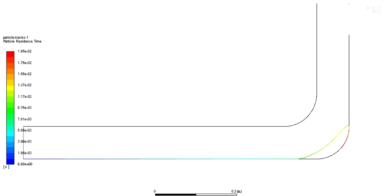
Figure 5.21: Particle tracking shows deposition of 1 \mu\text{m} diameter silica particles, as it separates from the free stream and reverses onto the outer wall.
