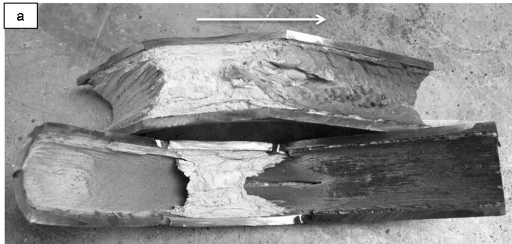
Figure 6.4: Erosion caused in the exit region of an outer bend retrieved from the geothermal flow experiment performed by Karlsdottir et al. (2014).
