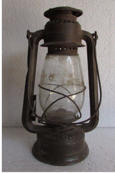
Figure 2.15: The soot layer covering the glass of an old kerosene lamp can be attributed to thermophoretic diffusion from the flame in the lamp.
