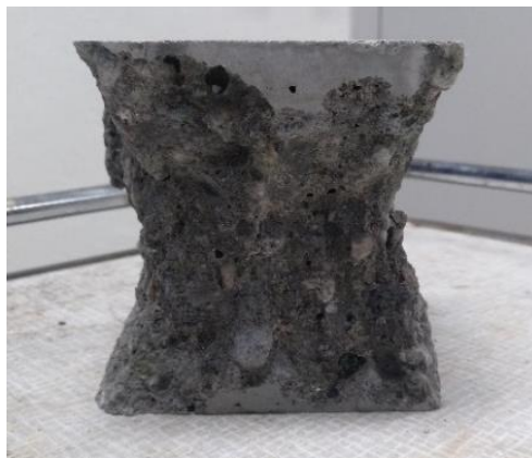
FIGURE 49: FRACTURED TEST SPECIMEN
