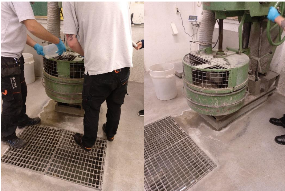
FIGURE 41: WET BLENDING PROCESS
