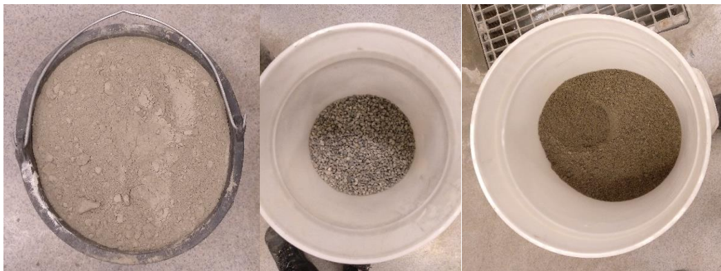
FIGURE 38: INGREDIENTS FOR THE CONCRETE MIX
