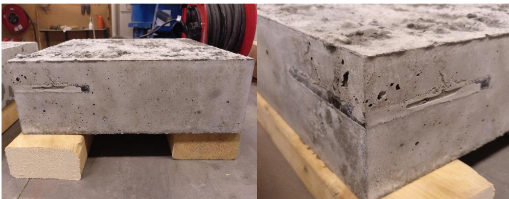
FIGURE 47: LATERAL VIEW AND DETAILED VIEW OF THE 30MM DEPTH SLAB
