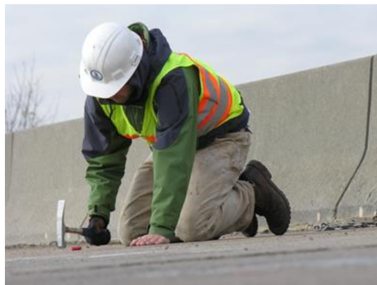
FIGURE 17: ACOUSTIC IMPACT TEST PERFORMED A WITH HAMMER [16]
