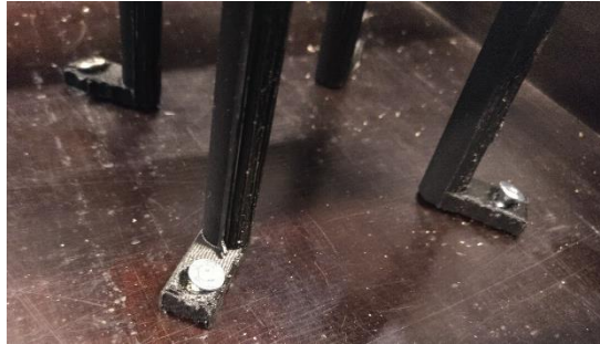
FIGURE 34: 3D PRINTED PART ATTACHED WITH SCREWS
