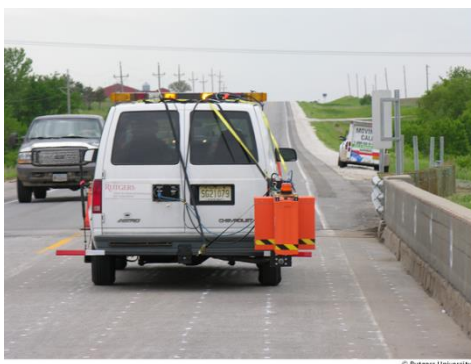
FIGURE 15: DATA ACQUISITION ON A BRIDGE DECK USING AIR-COUPLED GPR [15]
