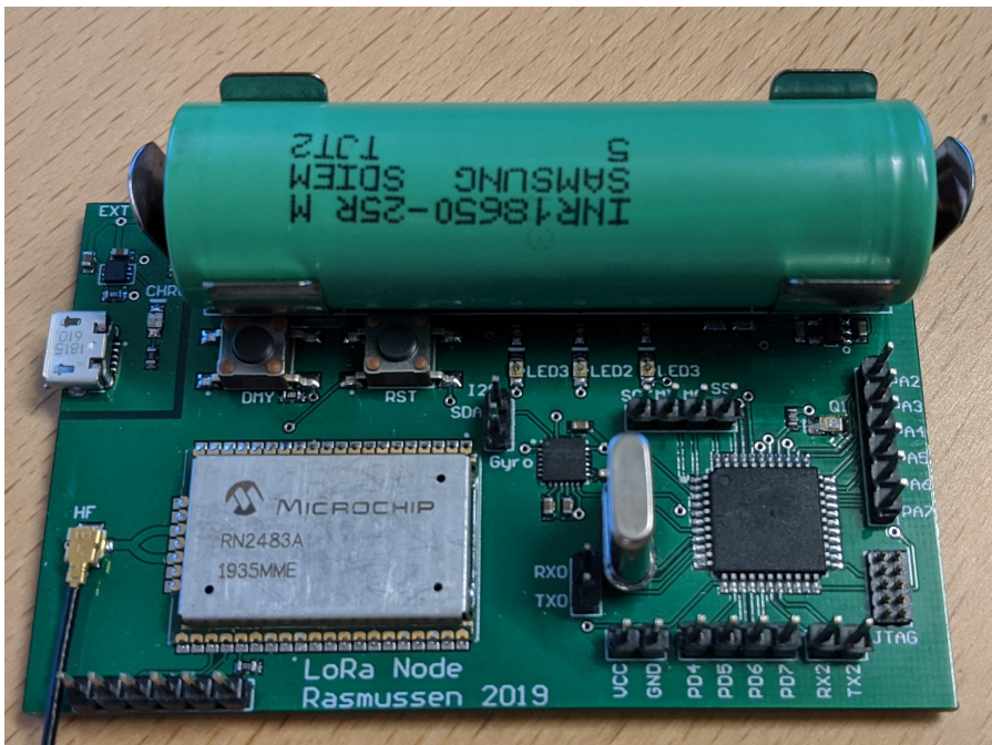
Figure 5.4: The assembled End-device with battery attached.
