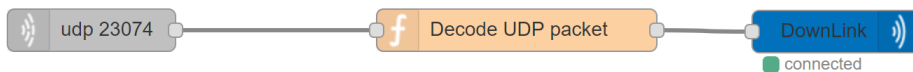
Figure 5.18: A snapshot of the code from the Node-RED application, showing the downlink-forward procedure.
