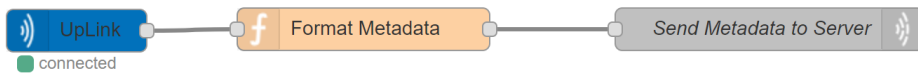
Figure 5.17: A snapshot of the code from the Node-RED application, showing the uplink-forward procedure.
