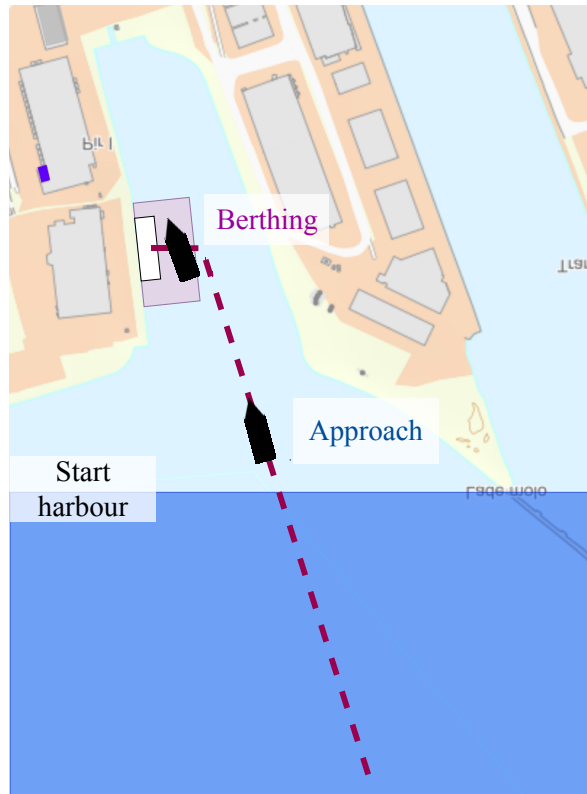
Figure 3.2: Illustration of the two phases, approach and berthing. The area outside the harbour is marked with a darker blue colour, while the harbour is the light blue and the purple area. The harbour has a speed limit of 2.5 m/s. The approach phase concerned both the darker blue and lighter blue areas, while berthing was performed in the purple area.
