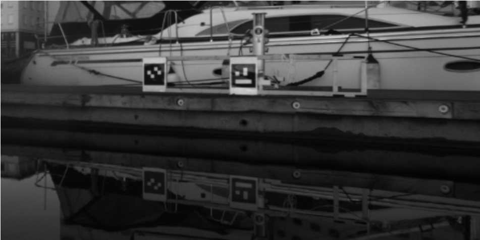
Figure 9.8: Reflection from water may confuse the detector. Specially the left marker can be challenging as it is nearly symmetric.
