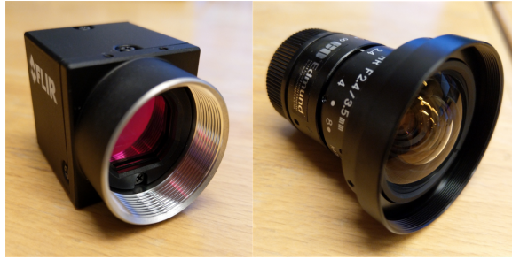
Figure 5.3: To the left, a FLIR Blackfly S GigE PoE machine vision camera. To the right, a wide angle lens from Edmund optics. Both are used throughout the master thesis.
