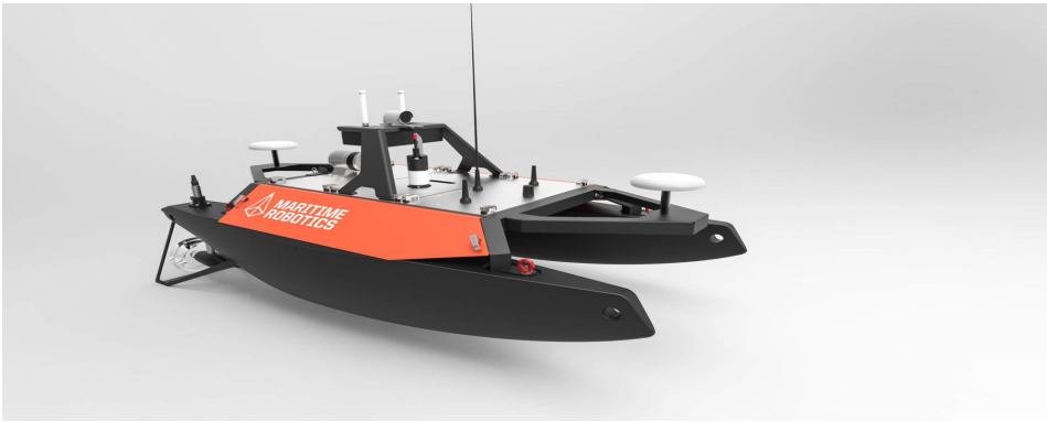
Figure 1.2: The Otter is a small and portable Unmanned Surface Vehicle (USV) suited for mapping and monitoring of its surroundings at sea. Image courtesy by Maritime Robotics [1].
