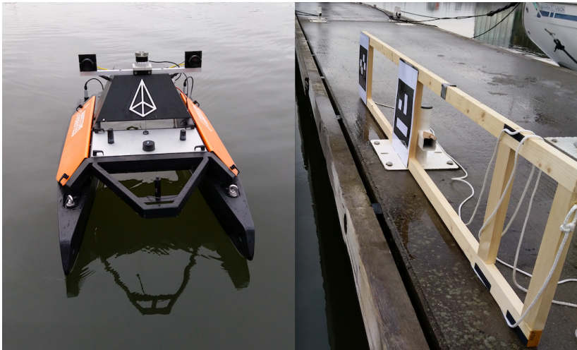
Figure 8.5: Visual shots of the two main components used during the experiments. To the left, the vision system armed on an Otter USV. To the right, the marker configuration used as the reference system to obtain position measurements.
