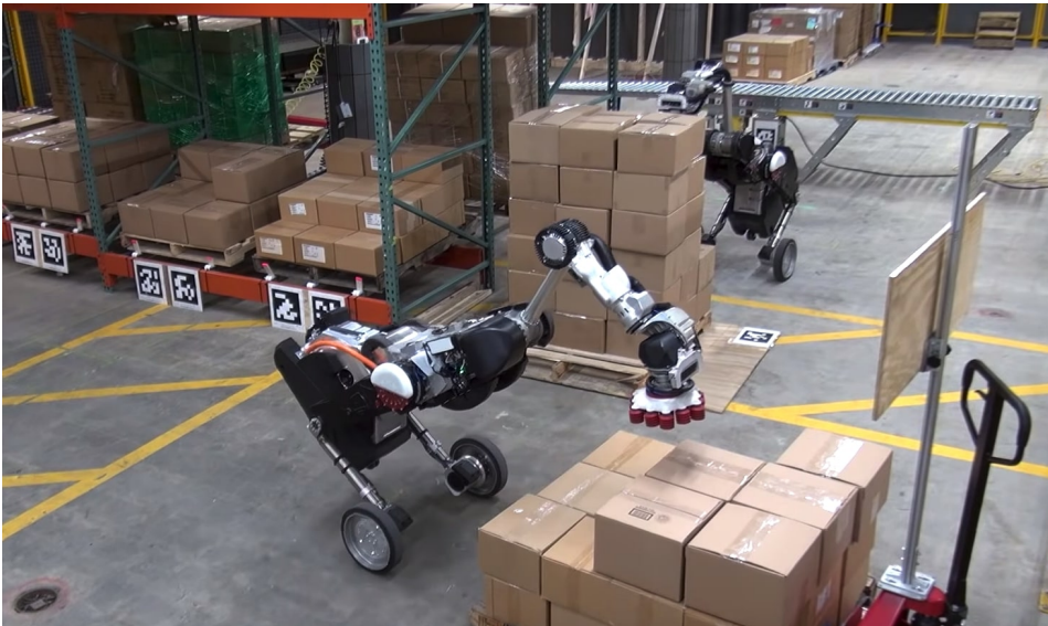
Figure 2.5: Boston Dynamics robot Handle combines depth cameras with ArUco markers to localize itself accurately and thereby handle different logistics tasks with a mobile manipulator. Image courtesy of Boston Dynamics [22].
