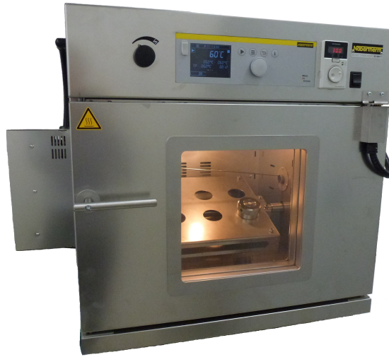
Figure 4.2: The digestion furnace used in the experiments, where mixing is achieved through swinging of a plane where the vessels are placed.
