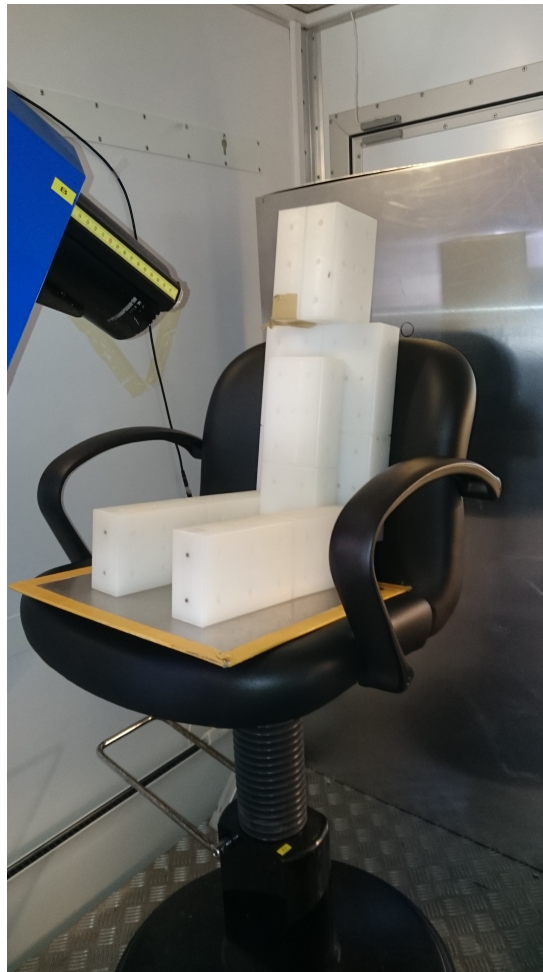
Figure 5.1: The smallest phantom, P_1 , during calibration. Detector holder, protection wall, plateau and chair visible. Small pins holds the phantom together.
