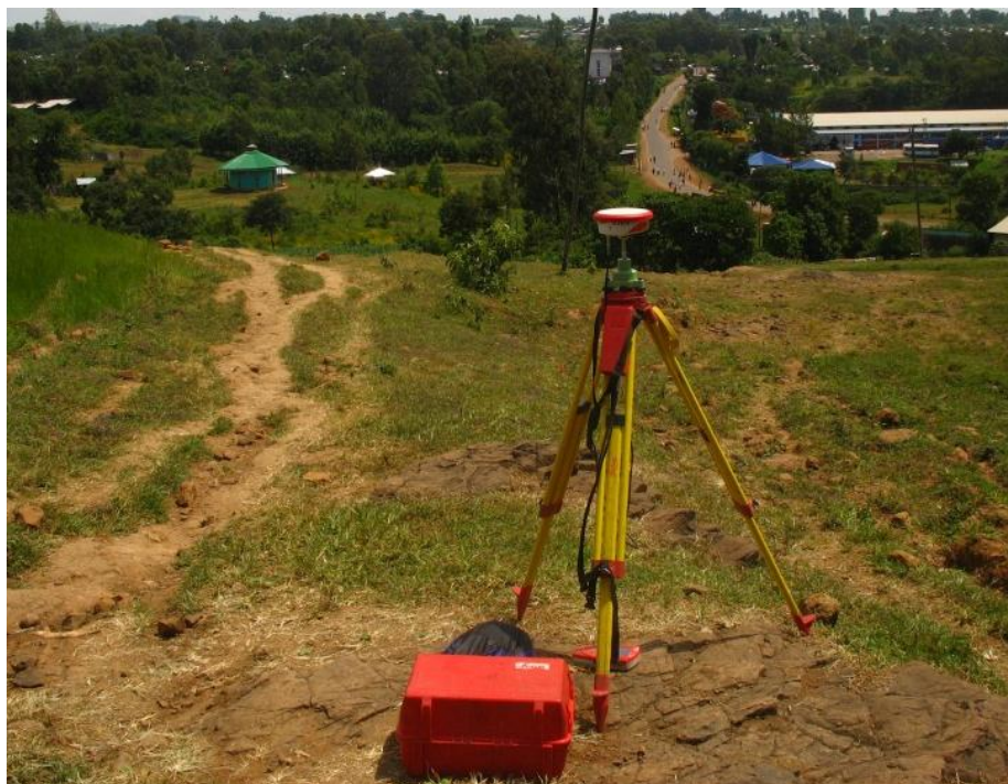
Fig. 13 Base station logging satellite positions in Bure.
