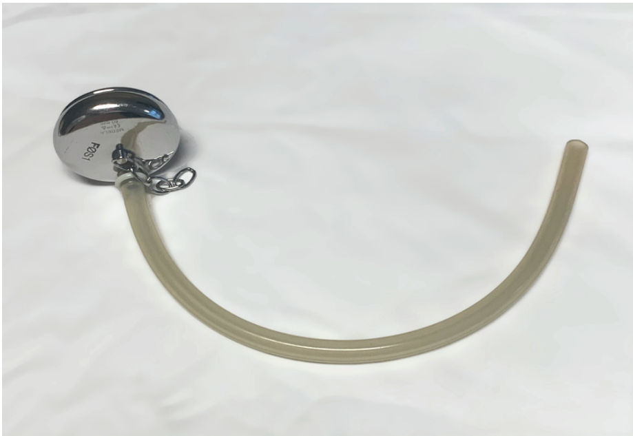
Figure 18. Malmstrom stainless-steel vacuum cup. Photo by Morten Dreier.
