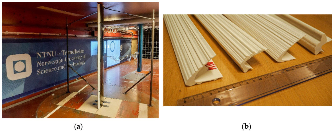
Figure 2. The wind tunnel set-up of the S826 consisting of dummy sections and the main part mounted vertically, with attached artificial ice shapes (a). The 3D printed ice shapes, from left to right: mixed, glaze, rime, and horn* (b).
