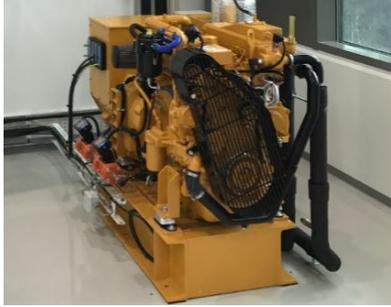
Fig. 1. The small marine diesel engine included in the hybrid power lab at the Department of Ocean Operations and Civil Engineering at the Norwegian University of Science and Technology in Aalesund.
