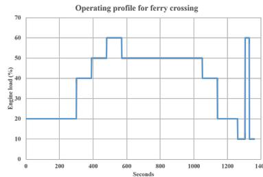
Fig. 2. Operating profile for a simulated autonomous ferry crossing.
