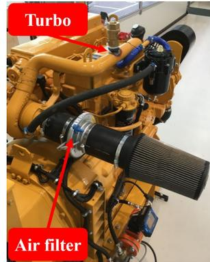
Fig. 4. The restriction and bleed device used to provoke the air filter and turbo fault, respectively.
