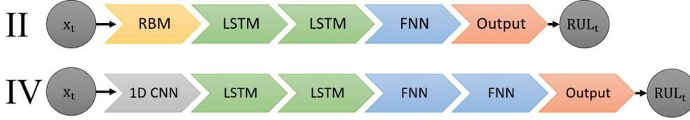
Figure 3.1: DNN structures proposed for the C-MAPSS data set [17, 22].
