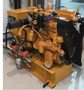
Fig. 2. The marine diesel engine included in the hybrid power lab.
