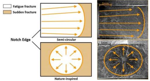
Figure 3: Different initiation sites for specimens with a variable radius (nature inspired) and specimens with a constant radius
