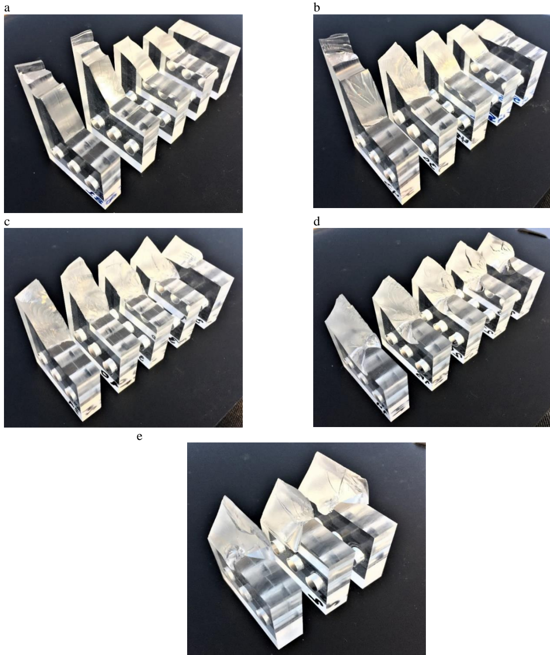
Fig. 16. CTS specimens fractured under different loading conditions, with \alpha=0^\circ on the right and \alpha=90^\circ on the left side of the pictures; (a) \beta=0^\circ , (b) \beta=22.5^\circ , (c) \beta=45^\circ , (d) \beta=67.5^\circ , (e) \beta=90^\circ .
