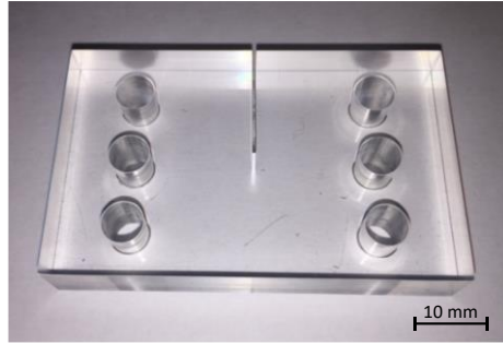
Fig. 11. A typical PMMA CTS test specimen.
