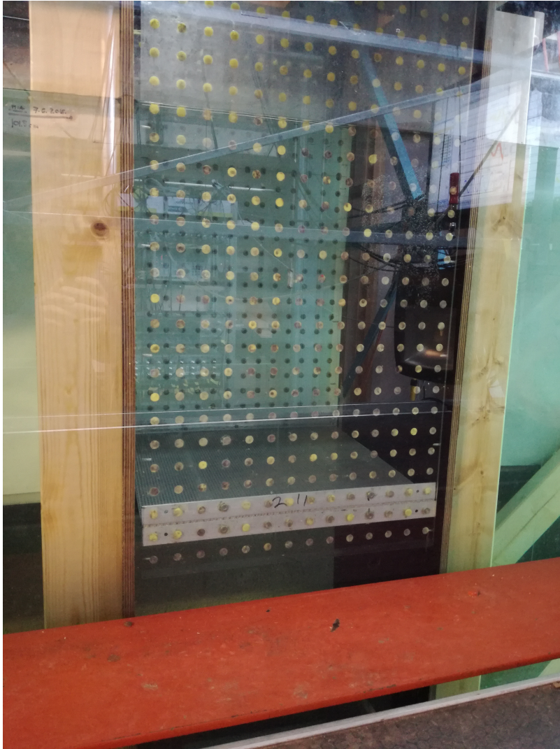
Figure 3.6: Forced oscillation experiments inside a channel. Generation of plate-end vortices is limited due to the small gap from the plate-end to the channel wall.
