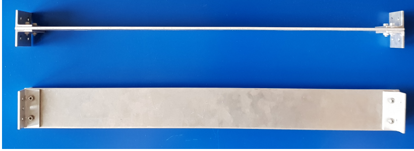
Figure 8.2: Side and top view of the experimentally tested plate. The plate is D = 60 mm wide, t = 4 mm thick ( \frac{D}{t} = 15 ) and has a lateral length of L = 570 mm. Photo by Frøydis Solaas.
