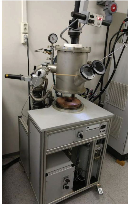
Fig. 3.3. Edmund Bühler AM/0.5 arc melter.
