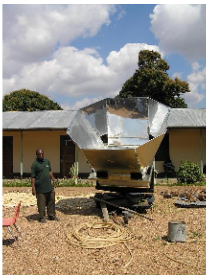
Figure 18 Village sized sun oven in the Catholic Sister's Camp in Masasi
