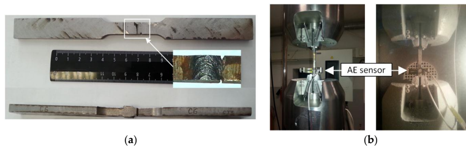
Figure 1. A view of the specimen. (a) A magnified image showing the weld joint and the notch shape. (b) Specimens mounted in the grips of the testing machine at 296 K (left) and 233 K inside the thermal chamber (right).
