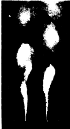
Figure 1.11: Helically forced jet, Re_D = 100\,000 , St_D = 0.27 . Adapted from Parekh et al. (1988).
