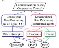
Fig. 2. Basic use of communication technologies for cooperative control. have concomitant access to the same communication link carrying the operational control references. Briefly, by relying on communication with a central agent as a fundamental part of the overall coordinated operation of inverters, the strategy can be defined as centralized.
