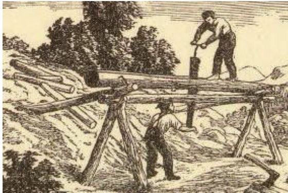
Figure 11. “The reflectiveness and permanent praxis of sawing logs by hand with a sawpit, developed the workmanship into craftsmanship/artistry” (Sundt, 1975, 213-214).
