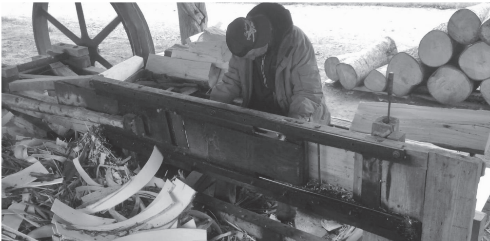
Figure 257. The old mechanical slicing of aspen shingles at the open-air museum in Samogitia (Photo taken by Giedrė Jarulaitienė, 2015).
