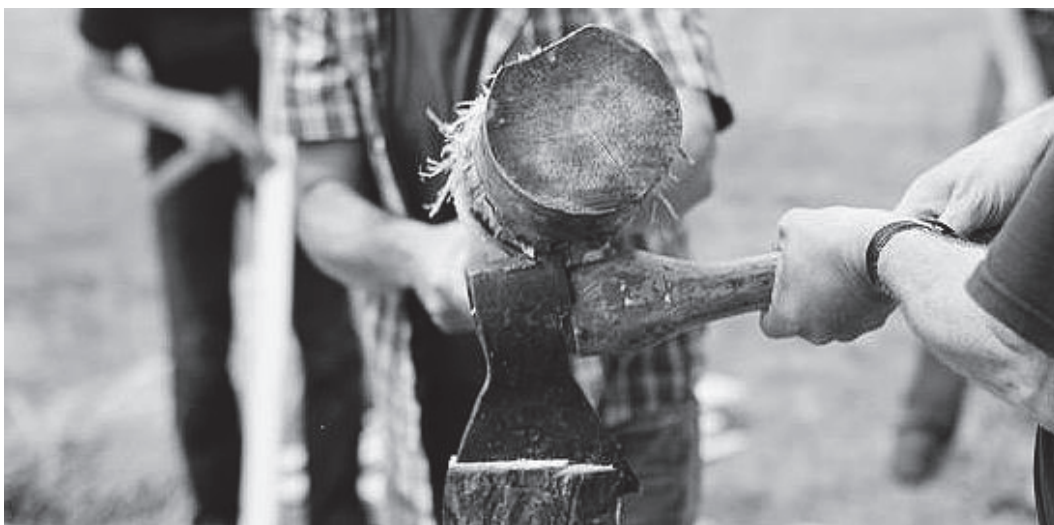
Figure 255. The hand-splitting of pine shingles ( dronyčios ) at the restoration workshop in one of the ethnographic villages in Dzūkija region (Photo taken by Giedrė Jarulaitienė, 2015).
