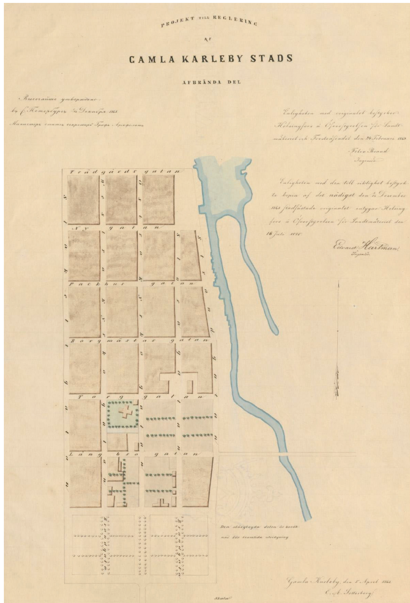
Figure 150. New fire breaks and guards were introduced in the main area of Kokkola in the 19th century according to the proposal of C. A. Setterberg (Projekt till Reglering Af Gamla Karleby Stads Afbrände Del. Planritningar öfver städerna i Finland, The National Archives of Finland).
