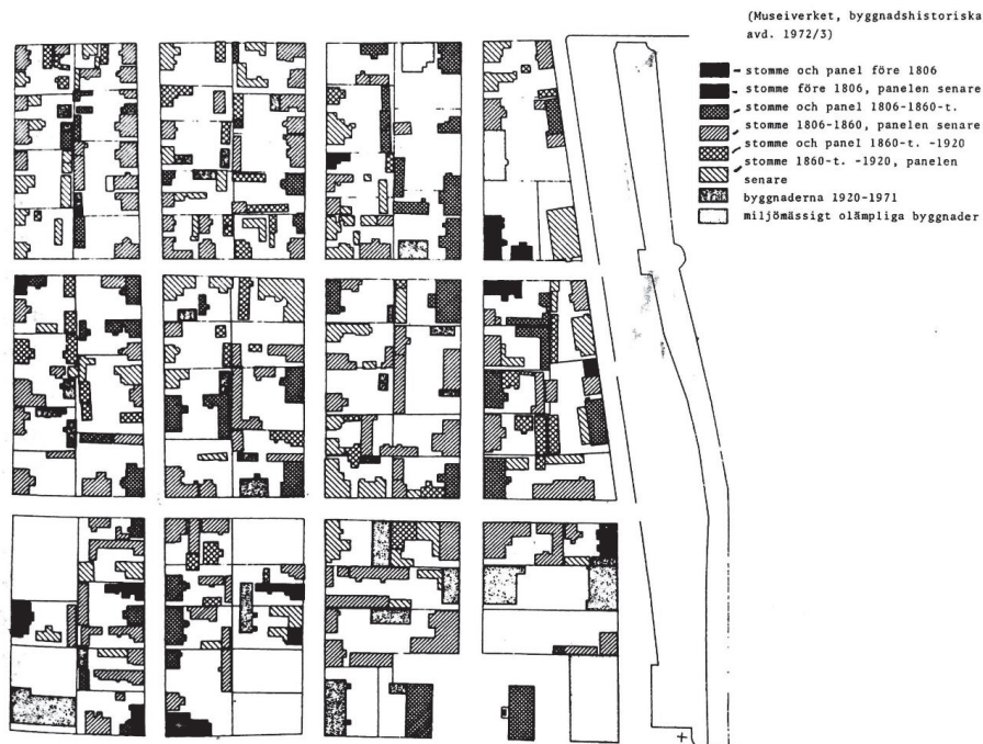
Figure 173. The inventory stock-taking, carried out by the Archeologic Commission in 1971, revealed the approximate dates when historical wooden buildings were built and transformed. The analysis also involved the evaluation of recent constructions, most of which were marked by a blank background on the map and described as “the environmentally-disadvantageous buildings” (Jalkanen et al., 1972, p. 11).
