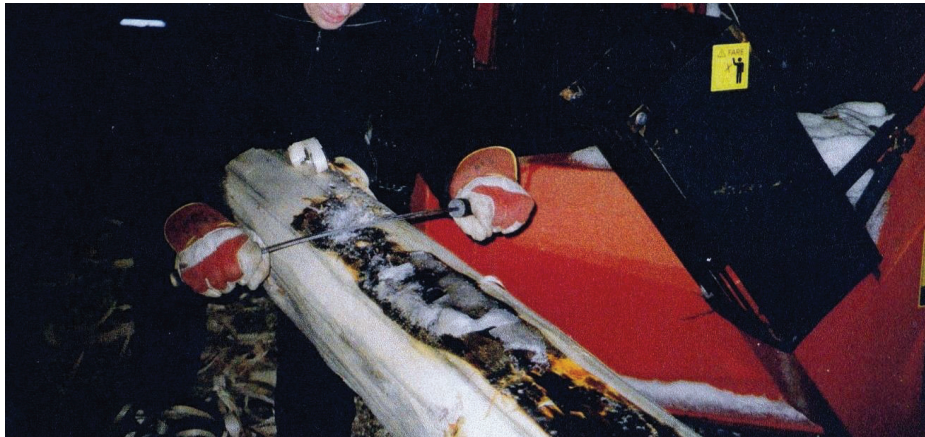
Figure 118. The manual debarking of logs at Nördalen in Os (The photographer unknown, 2009. The private archive of the carpenter).
