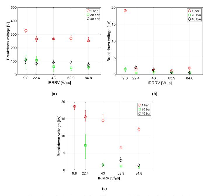
**Figure 6.** Breakdown voltage as a function of IRRRV for different filling pressures and at different electrode and nozzle configurations. (a) Free-burning arc. (b) Tube-constricted arc. (c) Self-blast arrangement. The scale of the Y axis is not same for three different configurations.
