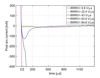
**Figure 8.** Post-arc current at 40 bar filling pressure in the self blast arrangement for different IRRRV.
