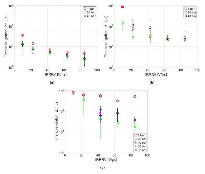
**Figure 5.** Re-ignition time as a function of IRRRV for different filling pressures and at different electrode and nozzle configurations. (a) Free-burning arc. (b) Tube constricted arc. (c) Self-blast arrangement.
