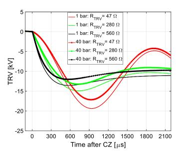
**Figure 2.** Influence of the arc voltage on the TRV shapes for different  $R_{\text{TRV}}$  s.
