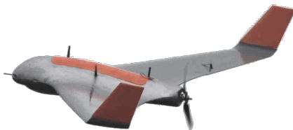
Figure A.2: Skywalker X8 sUAS - operated by AMOS UAVLab (Source: NTNU)
