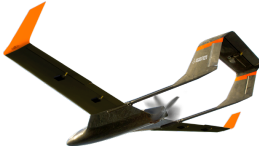
Figure 5.1: Maritime Robotics P31015 Prototype sUAS
