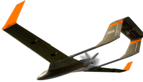
Figure 3.7: P31016 concept battery-powered fixed-wing unmanned aircraft
