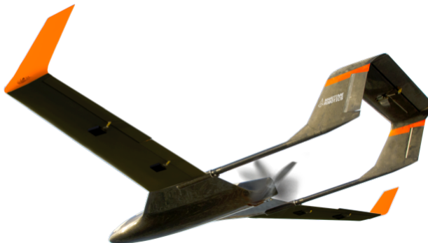
Figure 2.4: P31016 concept battery-powered fixed-wing unmanned aircraft
