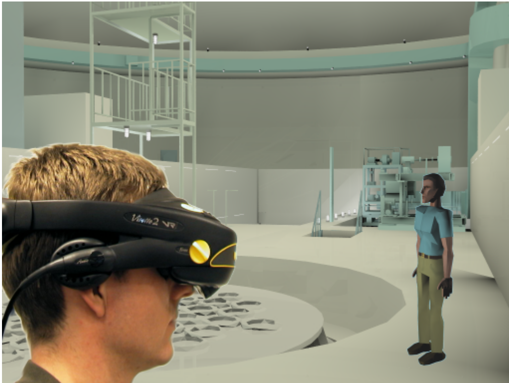
Figure 14. Example of VE used for field operation. Field operation simulation in VR gives the opportunity to simulate situations where the field operator is prevented from doing his job by physical or organisation constraints. The person wearing the HMD can see his colleague in the virtual environment.
