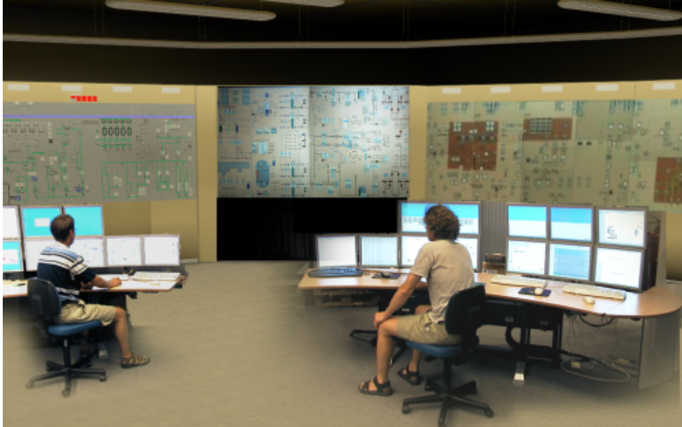
Figure 12. Manipulated picture from HAMMLAB where the turbine operator (to the right) works together with a manikin reactor operator in the situations where operation and monitoring of control panels are necessary.
