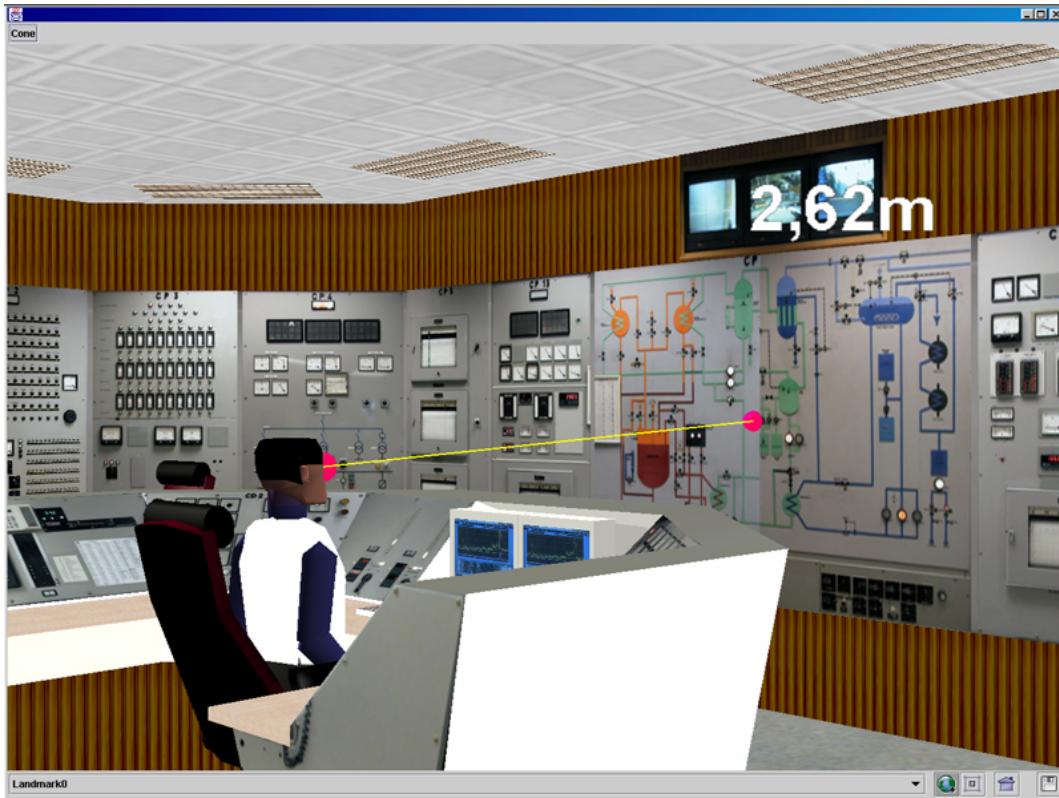
Figure 3. Screen dump of measurement in the VR condition. The length of line drawn from the manikin's head to the control panel (2,62 meters) is displayed in the upper right part of the figure.
