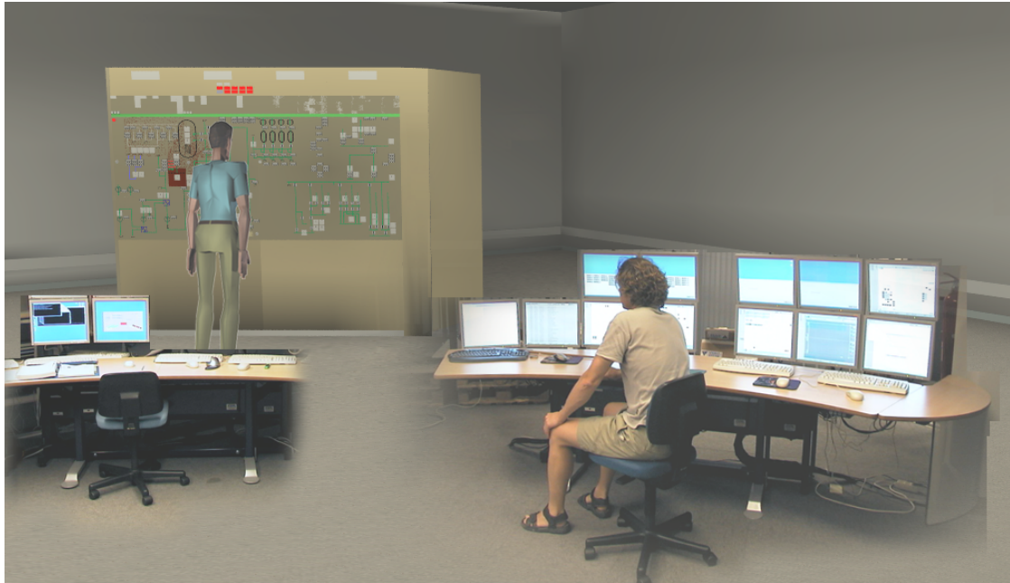
Figure 7. Manipulated picture from HAMMLAB where a VR model is used to represent the conventional panels on the reactor side.
