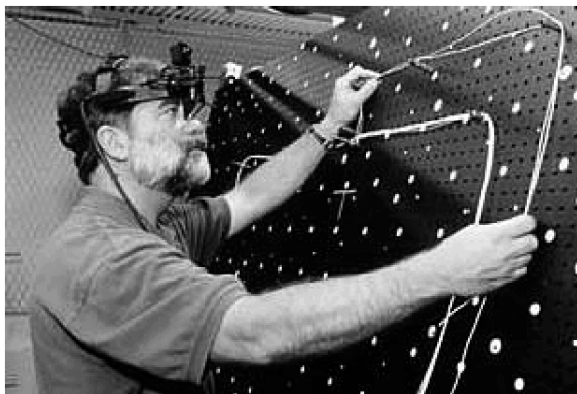
Figure 3. A prototype wire harness assembly system developed by Boeing.
