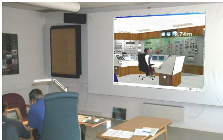
Figure 2. Experimental set-up in the VR condition: The subject is placed in front of a screen showing the projection of the VR model.
