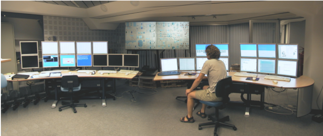
Figure 6. Picture from the HAMMLAB with the reactor operator control station to the left and the turbine operator control station to the right. A large screen is placed between the two control stations.
