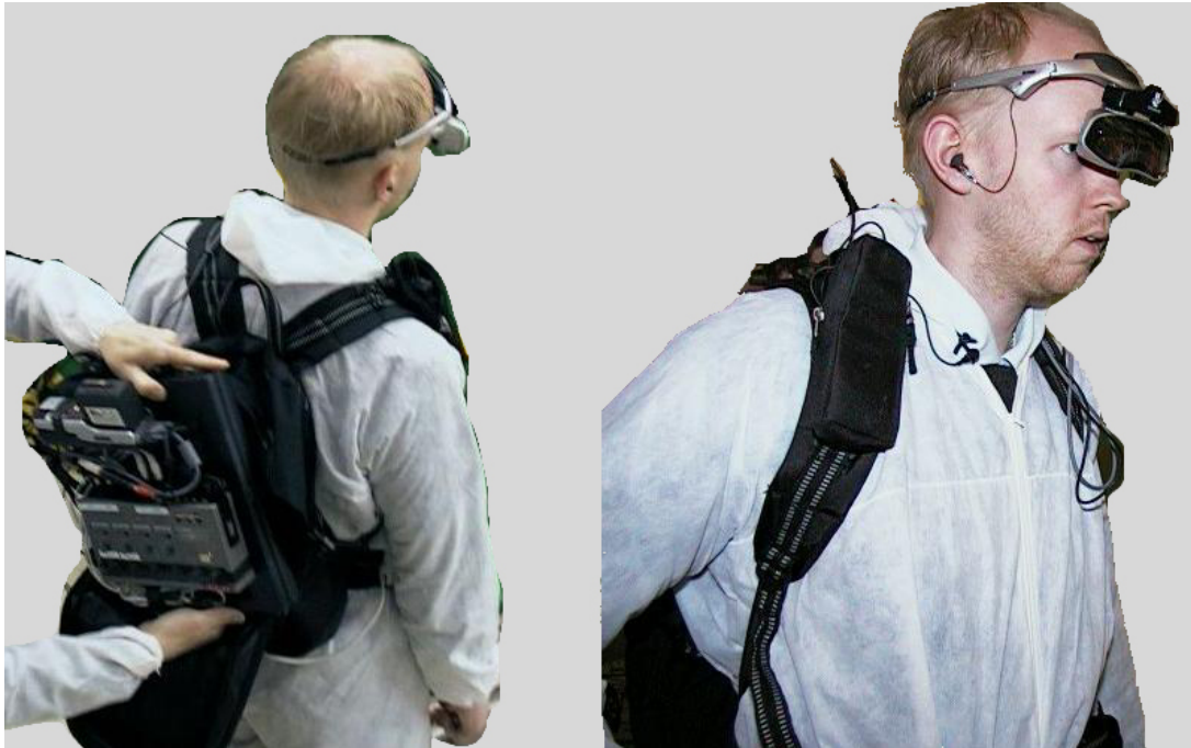
Figure 6. The figure shows the wearable equipment consisting of a laptop in a backpack and a HMD with integrated audio. The head-orientation tracker is mounted on top of the HMD's display unit.
