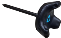
Fig. 8. Simple tool based on a Vive Tracker with a 15 cm long and 1 cm thick spike probe screwed into its quarter inch UNC threaded camera mount.
