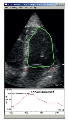
Fig. 4. Example segmentation from a PSU recording. The circles in the basal region of the model correspond to  $\mathbf{p}_{i,K}$  and the circles in the myocardium correspond to  $\mathbf{x}_{i,S}$ .
