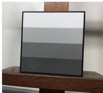
Figure 2. Multi-step reflectance standard with reflectances at 99%, 50%, 25% and 12.5%
