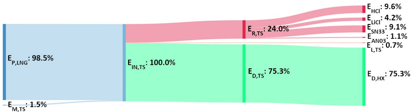
Fig. 9. Exergy flows for the thermal storage central plant
