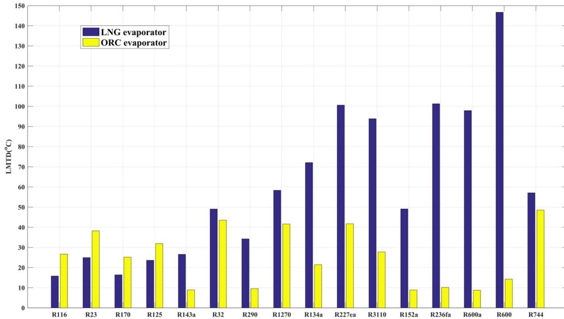
Fig. 6 LMTD for LNG and ORC evaporators in CODW
