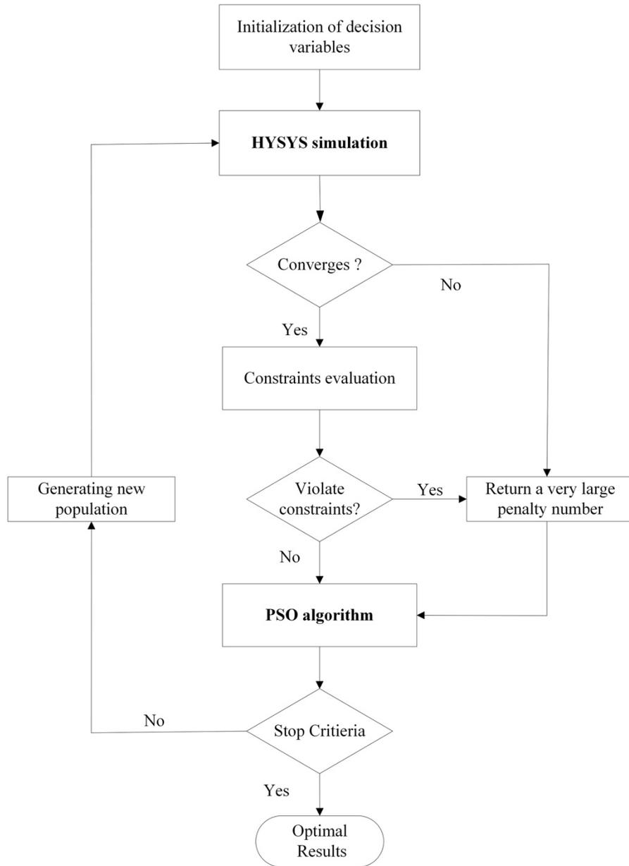
Fig. 3 Simulation-based optimization framework
