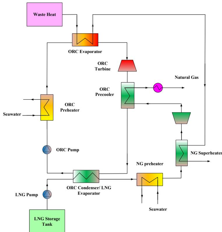
13 Fig. 2 The flowsheet of the Combined ORC and DE with Waste heat utilization (**CODW**)
