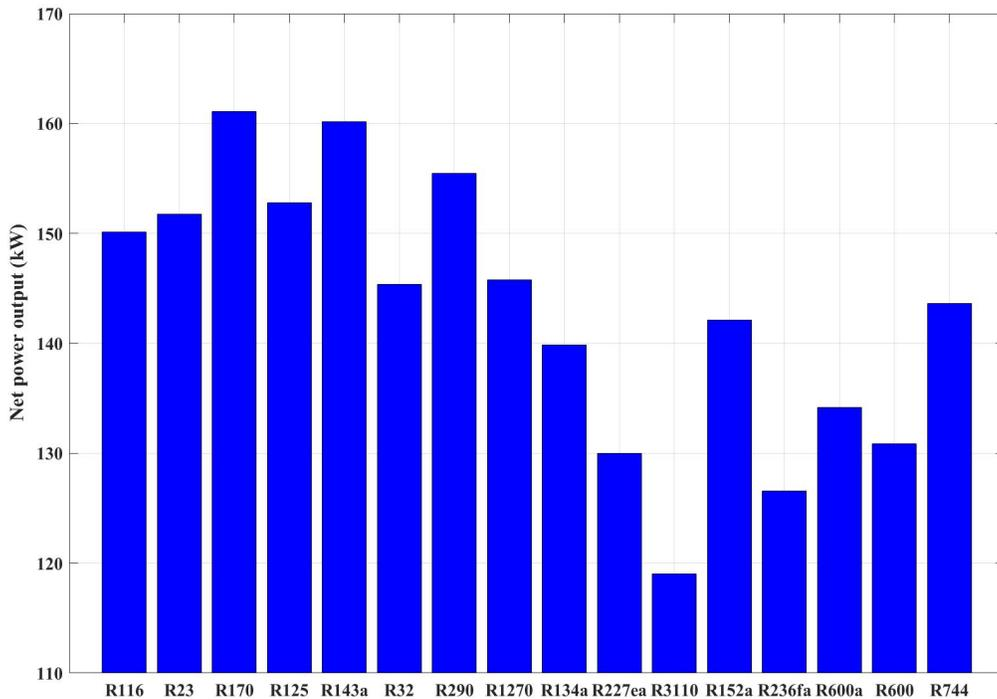
Fig. 5 Power output of working fluids in CODW
