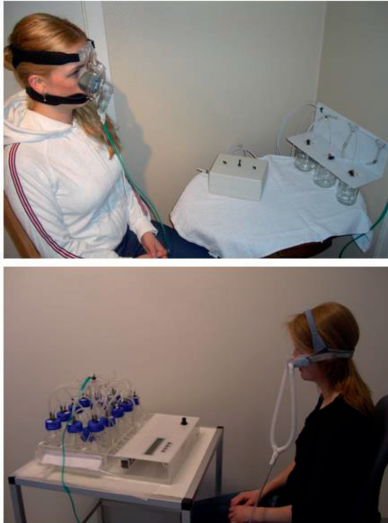
Figure 6. Images of the two olfactometers produced for this project. The manually-controlled olfactometer used in study III is shown in the upper image. The automatically-controlled olfactometer is shown in the lower image and was used in an fMRI experiment not included in this thesis.
