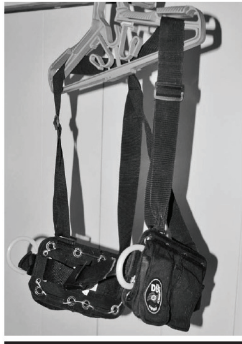
FIGURE 3. DUI weight and trim system with bilaterally removable weight pockets (by pulling surgical tubing loops) and shoulder harness.
