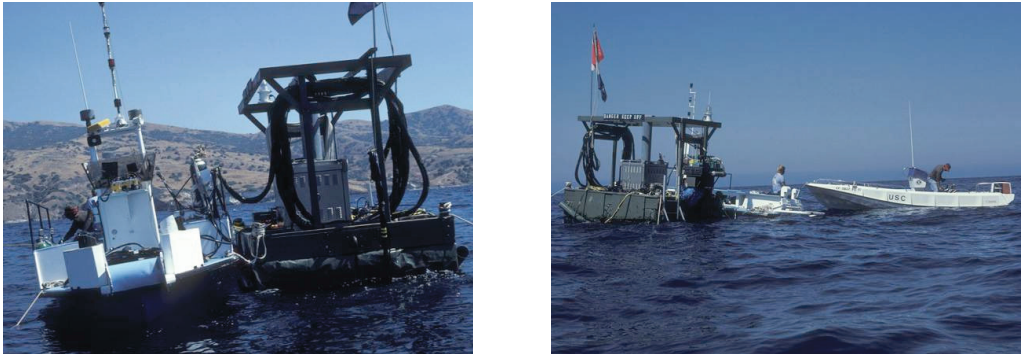
Figure 6. Tender boat and support barge with hot water and compressed air supply.
