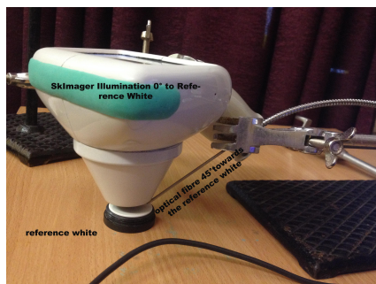
Figure 2. Measurement setup to measure the spectral power distribution of the LEDs in the SkImager with a 0^\circ/45^\circ measurement setup according to the CIE 3
