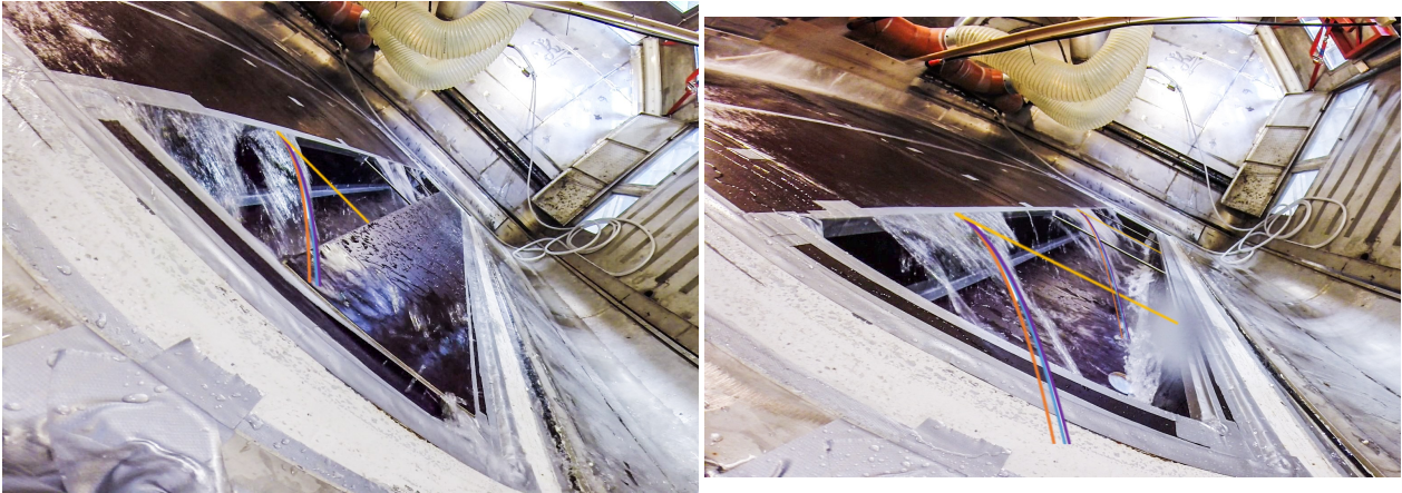
(a) 240mm gutter opening in comparison to experiment
