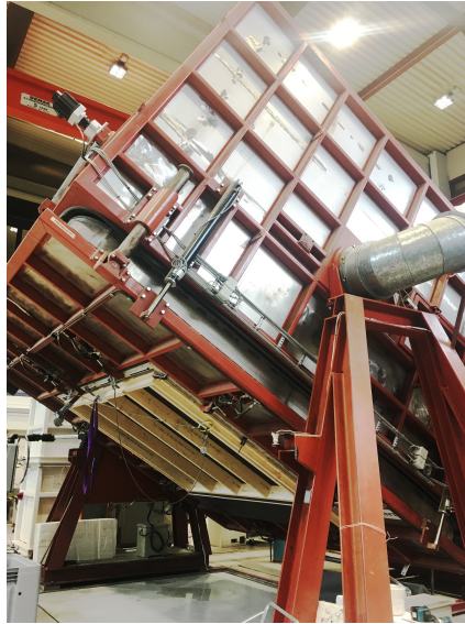
Figure 2.8: Rain and Wind (RAWI) Box at SINTEF Laboratory
