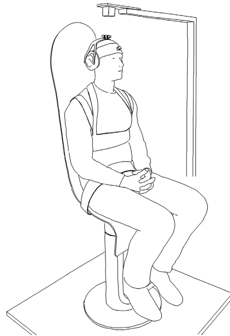
Figure 1. An instrumented subject strapped to the actuated chair. The cube above the subject's head represents the electromagnetic transmitter. Note that the ear muffs have holes leaving the ears uncovered to enable communication with the subject and not induce further modulation of sensory input with potentially unknown effect.
