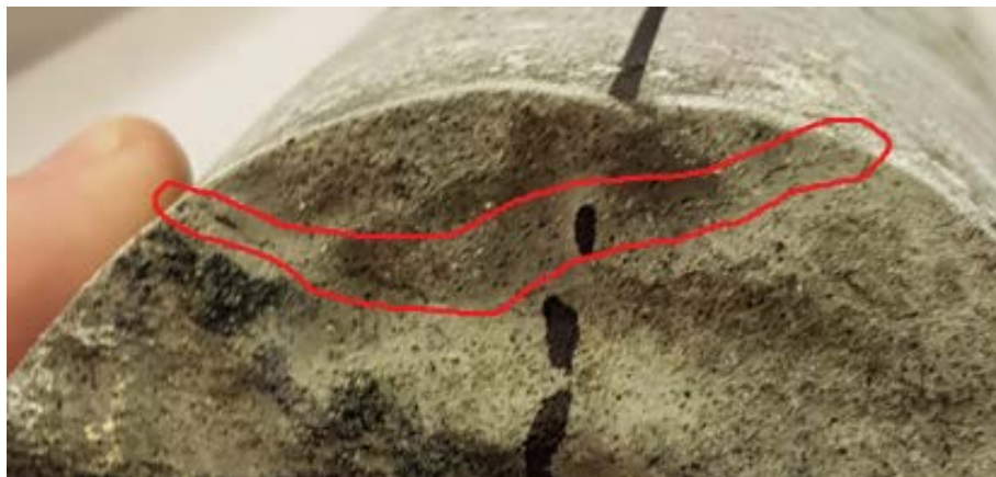
Figure 4-15 Core M6 with a crack
