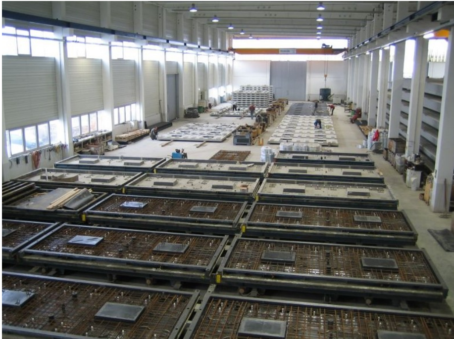
Figure 56 Production facility with steel moulds (PORR Bau GmbH, 2016)
