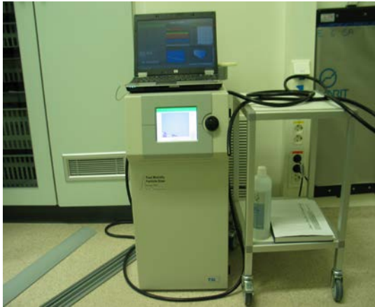
Figure 2-5. The FSMP Spectrometer Model 3091 placed by the wall in the operating room. The picture was taken before an operation during the study.
