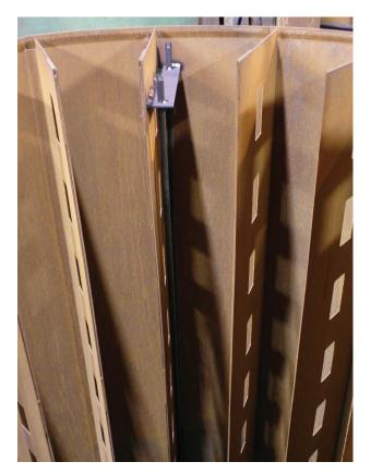
Figure 3-6: The steel tubes for thermocouples 7 and 8 attached to the fin of the electrode casing
