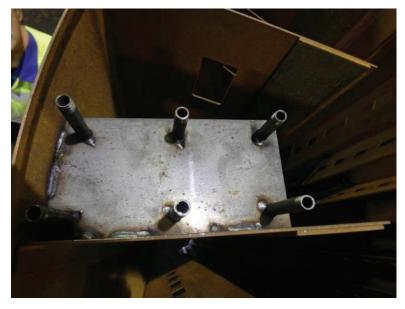
Figure 3-5: A picture of the tubes for thermocouples 1-6. The large steel plate used to hold the tubes in place was not recommended by the author. Less steel should have been used to have a more continuous carbon electrode in this area.
