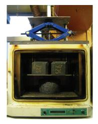
Figure 4-4: The furnace for flow measurements with sample inside.
