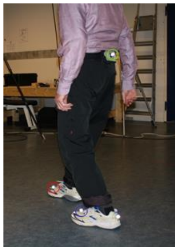
Figure 1. Marker set-up. Red circle: toe marker right foot, blue circle: toe marker left foot, green circle: lumbar marker.
