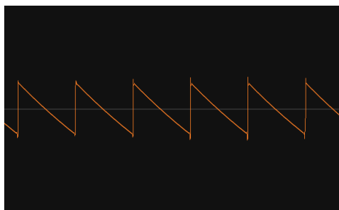
Figure 2.4: A saw wave in the time domain. Voltage as a function of time.
