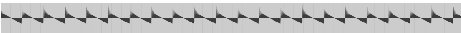
Figure 4.14: A short slice of the saw wave affected by a low pass filter.
