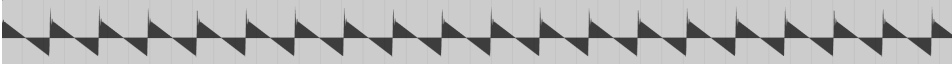
Figure 4.16: A short slice of the saw wave affected by a low pass filter with changing resonance.
