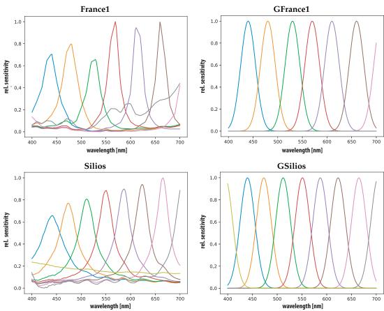
Figure 3. Sensor sensitivities, one RGB camera [60], a prototypical implementation by Thomas et al. [3] (France1) and commercially available Silios [6] (Silios) (all left) and simulated GSB (GRGB, GFrance1 and GSilios) versions (all right).
