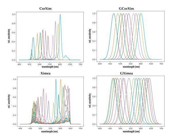
**Figure 4.** Sensor sensitivities, Ximea xispec [4] (Ximea and CorXim) (all **left**) and simulated GSB (GCorXim and GXimea) versions (all **right**).
