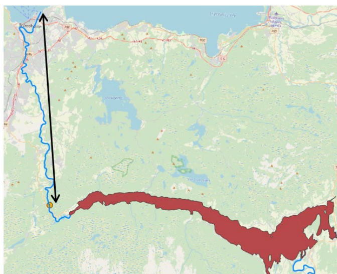
Figure 3.15. Selbusjøen (red shape) and the blocking of access to the fjord. River Nidelva (blue line) flows out of Selbusjøen to the fjord in the North and the orange circle represents the dam of Selbusjøen.
