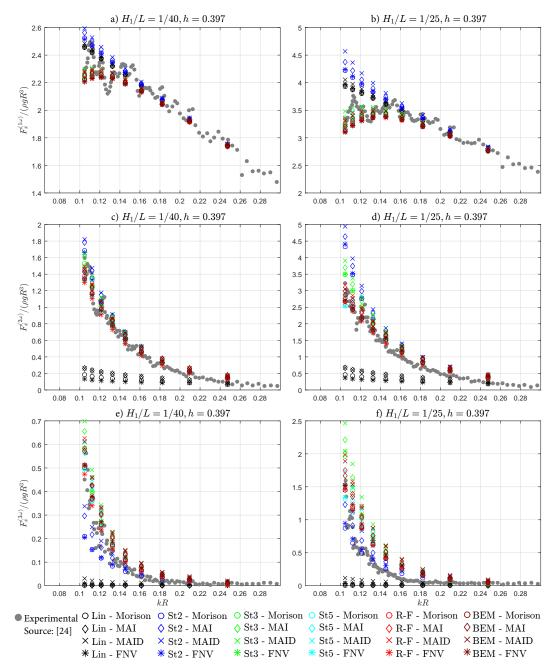
**Figure 10.** First (**a**–**b**), second (**c**–**d**) and third (**e**–**f**) harmonics of the normalized horizontal force over the increasing wave number kR for two steepnesses of  $H_1/\lambda = 1/40$  (**a**,**c**,**e**) and  $H_1/\lambda = 1/25$  (**b**,**d**,**f**) for the depth h = 0.397 m, compared with experiments from [24] (grey dots).
