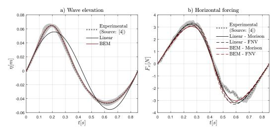
**Figure 4.** Comparison of a selection of computed: (a) wave elevation profiles, (b) loading models, with the superimposed experimental measurements reported in Grue and Huseby (2002) [4], for the case with wave steepness kH/2 = 0.31 and wave period T = 0.85 s (error bars are the standard deviation from the superimposition at zero-upcrossings).
