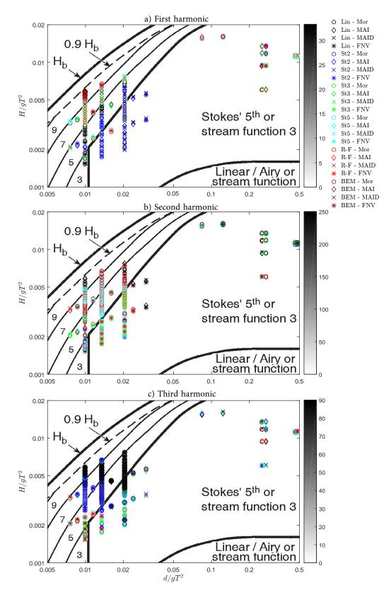
**Figure 12.** The three best-fitting numerical models for the first (**a**), second (**b**) and third (**c**) harmonics with the intensity behind the symbol referring to the relative error (the darker—the worse the error, scale dependent on the harmonic), displayed on the wave theory limit graph from [34].  $H_b$  stands for the breaking wave limit. Marker color denotes the wave kinematics, marker symbol—hydrodynamic loading model. For reference to experiments see Figure 3.
