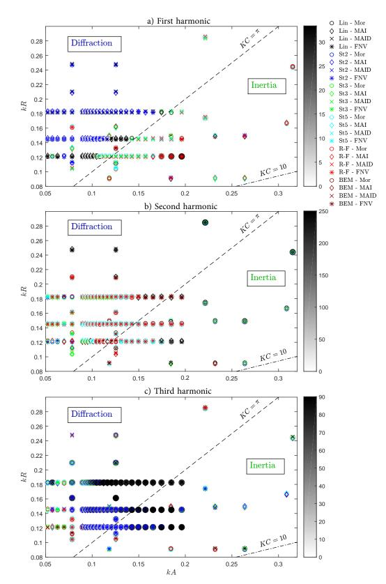
**Figure 11.** The best-fitting numerical models for the first (**a**), second (**b**) and third (**c**) harmonics with the intensity behind the symbol referring to the relative error (the darker—the worse the error, scale dependent on the harmonic), displayed on (kA, kR)-grid. Marker color denotes the wave kinematics, marker symbol—hydrodynamic loading model. For reference to experiments see Figure 2.
