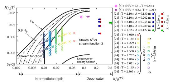
**Figure 3.** Experimental studies analyzed in this paper with reference to the limitations of regular wave theories as defined by IEC 61400-3 Design requirements for offshore wind turbines [34].  $H_b$  denotes the wave height corresponding to the wave-breaking limit. Identical markers in the Kristiansen and Faltinsen (2017) [24] cases refer to cases with increasing steepness for the same wave period and water depth.
