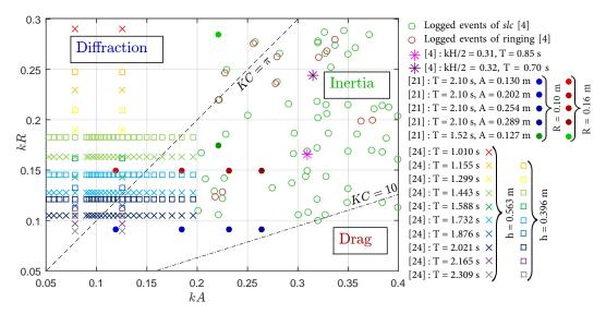
**Figure 2.** Experimental studies analyzed in this paper, on a (kA, kR)-grid, with reference to historically observed secondary load cycles as reported in Grue and Huseby (2002) [4] and the diffraction, inertia and drag regimes separated by the *KC* number equal to  $\pi$  and 10. Identical markers in the Kristiansen and Faltinsen (2017) [24] cases refer to cases with increasing steepness for the same wave period and water depth.
