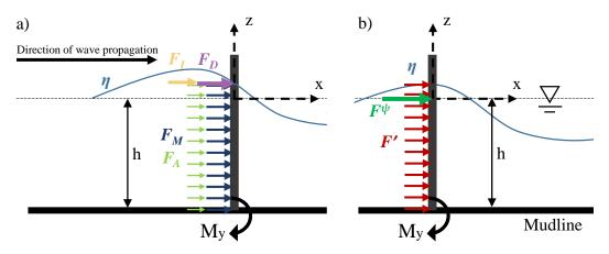
**Figure 1.** Coordinate system and the implemented hydrodynamic loading model components of: (a) Morison equation (integrated inertia term  $F_M$ ) and Rainey theory (integrated terms  $F_M + F_A$ , and point loads at the instantaneous free surface  $F_I + F_D$ ); (b) FNV theory (integrated term F' and point load at mean water level  $F^{\psi}$ ).
