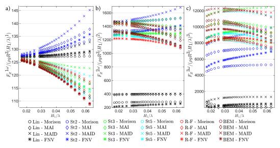
**Figure 6.** First (**a**), second (**b**) and third (**c**) harmonics of the normalized horizontal force over the increasing wave steepness  $H_1/\lambda$ . Corresponds to the experimental cases by Kristiansen and Faltinsen (2017) [24] with T = 2.021 s in the depth h = 0.564 m.
