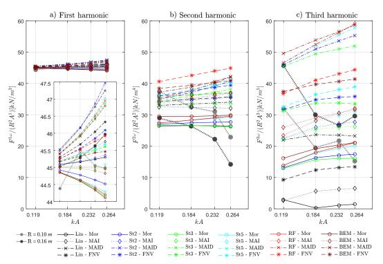
**Figure 8.** First (**a**), second (**b**) and third (**c**) harmonics of the normalized horizontal force over increasing steepness kA with period T = 2.10 s. Comparison between the experimental results from Stansberg (1997) [21] and numerical loading models. The y-axes are fixed to the same values for easier comparison, therefore a zoom of the first harmonic is provided in panel (**a**).
