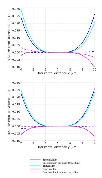
Figure 3. Model ISO: Relative error in traveltime for different extrapolation approaches along the lines y = 5 km (top) and x = 7 km (bottom).
