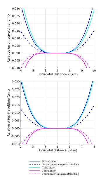
Figure 9. Model VTI: Relative error in traveltime for different extrapolation approaches along the lines y = 5 km (top) and x = 7 km (bottom).
