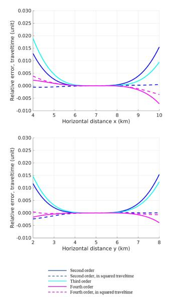
Figure 6. Model VEL: Relative error in traveltime for different extrapolation approaches along the lines y = 5 km (top) and x = 7 km (bottom).
