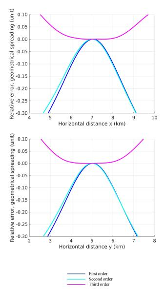
Figure 10. Model VTI: relative error in geometrical spreading for different extrapolation approaches along the lines y = 5 km (top) and x = 7 km (bottom).
