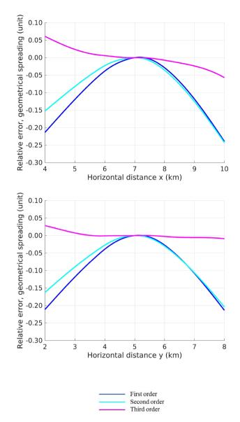
Figure 7. Model VEL: relative error in geometrical spreading for different extrapolation approaches along the lines y = 5 km (top) and x = 7 km (bottom).
