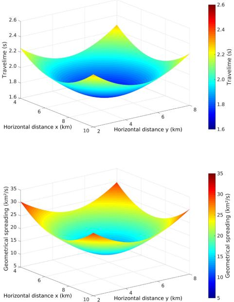
Figure 8. Model VTI: ray-tracing simulated P-wave traveltime (top) and geometrical spreading (bottom) in the plane at depth 0 km for a source point at depth
