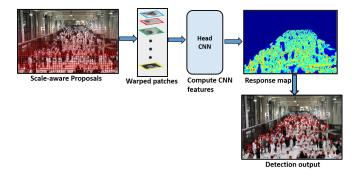
**Fig. 1**. Pipeline of Density Independent and Scale Aware Model (DISAM).
