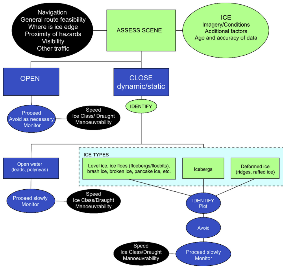
Fig. 1. An example of a human decision process when transiting in ice, adapted from Snider [1]; p. 88–89 with some modifications to highlight (in green) the importance of ice identification when transiting in ice.
